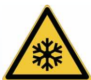
W010 - Warning: Low temperature/freezing conditions
