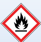
GHS 02 Flammable Self-reactive Pyrophoric liquids & solids Self-heating reactive Emit flammable gases Organic Peroxides
