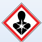
GHS 08 Respiratory sensitisation Germ cell mutagenicity Carcinogenicity Reproductive toxicity Specific Target Organ Aspiration hazard
